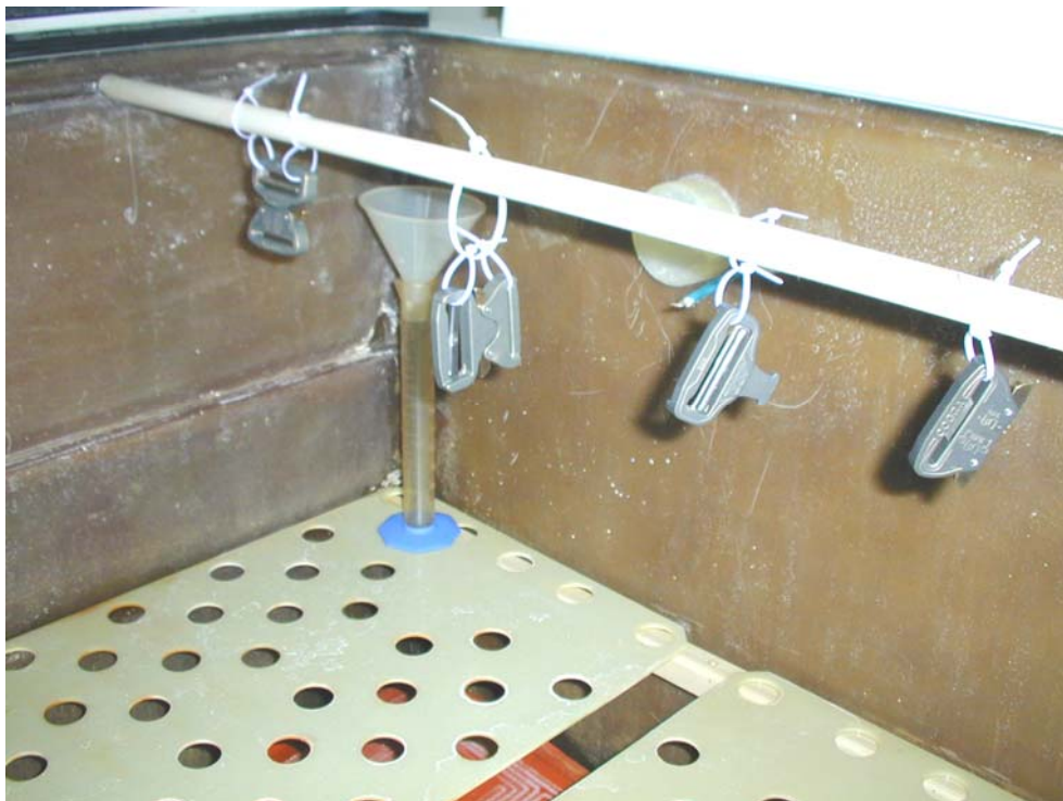
Photograph 2: Test units placed in salt fog chamber
