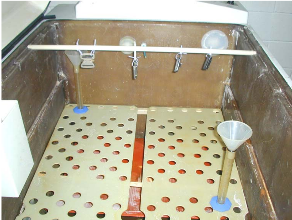
Photograph 1: Test units placed in salt fog chamber
